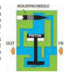
When inlet pressure is removed, downstream air is exhausted through the inlet port and around the point of the adjusting needle.
