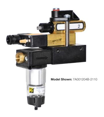
The electronically controlled multiple-point lubricator has a 3-way solenoid-controlled valve to produce the actuating signals for the Servo-Meters (up to four may be used.). This allows lubrication control to be interfaced with other system electronics, so that the frequency of oil injection is under precise control.
