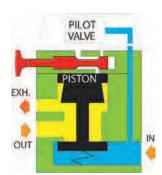
With solenoid pilot de-energized the inlet poppet is always closed. Downstream air pressure is exhausted via the exhaust port.
