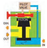
With the lockout handle pushed inward air to the piston is cut off. The inlet poppet closes, and downstream air pressure is exhausted via the exhaust port.
