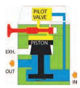
With solenoid pilot energized and the lockout handle pulled outward, pressure on the piston opens the inlet poppet and air flows freely from inlet to outlet. The exhaust port is closed.
