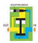
When downstreaam air pressure reaches the range of 40% to 60% of inlet pressure, the valve element shifts to the full open position and there is full air flow to the downstream components. This condition continues as long as there is air pressure at the inlet.
