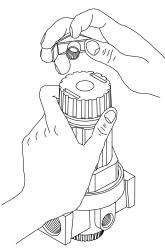
All vanguard high capacity series regulators are standard with locking knobs. A "key" is pushed in to adjust the regulator. When pulled out, the adjusting knob spins freely. Pried up on one end, the key is removed as shown and the regulator setting is tamper resistant.
